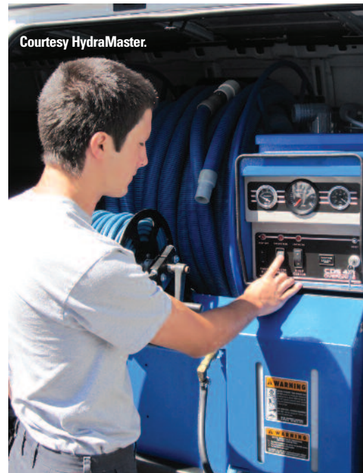
It's important to completely circulate the antifreeze solution to properly protect all machine components.
